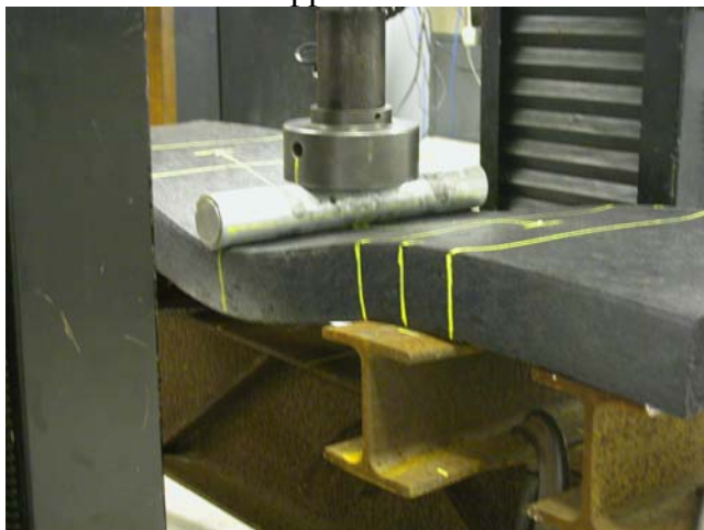
4300# load on 20" beam centers.
