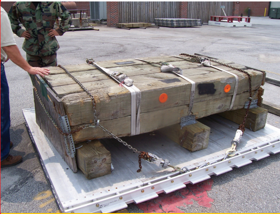
EXAMPLE OF THE WOODEN COMBAT OFFLOAD PALLET USED PRIOR TO RUMBER'S COP.
